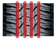
4 Main Straight Grooves for drainage performance, antiaquaplaning capabilities and to support wet braking.
