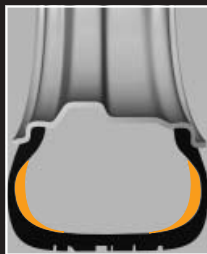
SSR runflat tyres The stable sidewalls support the tyre if it loses air.
